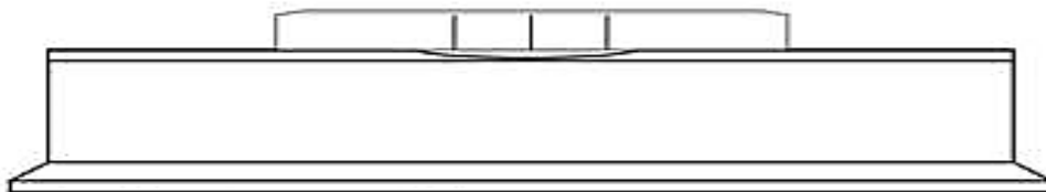
Figure SUB-PART D – 32 – Localized Surface Collapse
