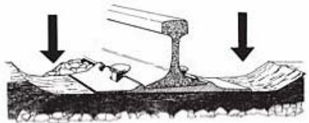
Tie Adzed to a Depth of 2" or Greater
